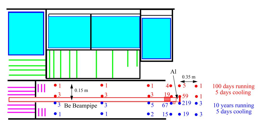
Dose rates in µSv/h from the Pixels+SCT+TRT+LAr cal.+VI beampipe after 10 years of running and 5 days cooling. Calculation by M. Morev.
