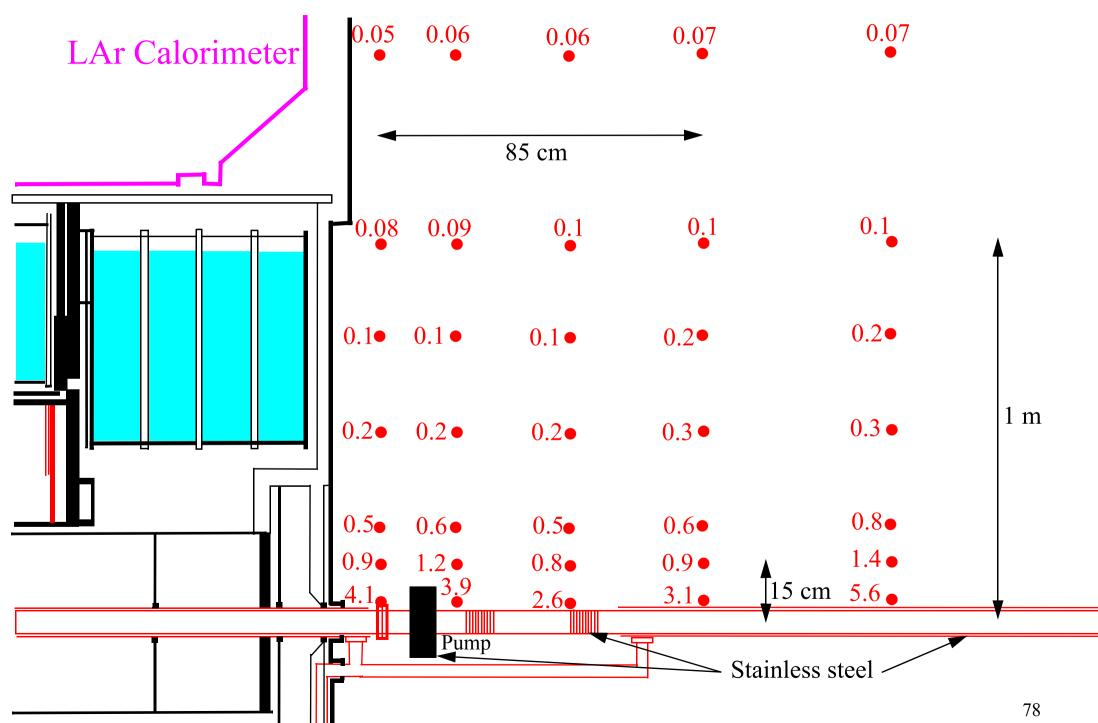
Dose rates in mSv/h from the VA beampipe after 10 years running and 5 days cooling.
