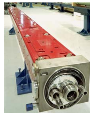
One of the superconducting dipole bending magnets.
