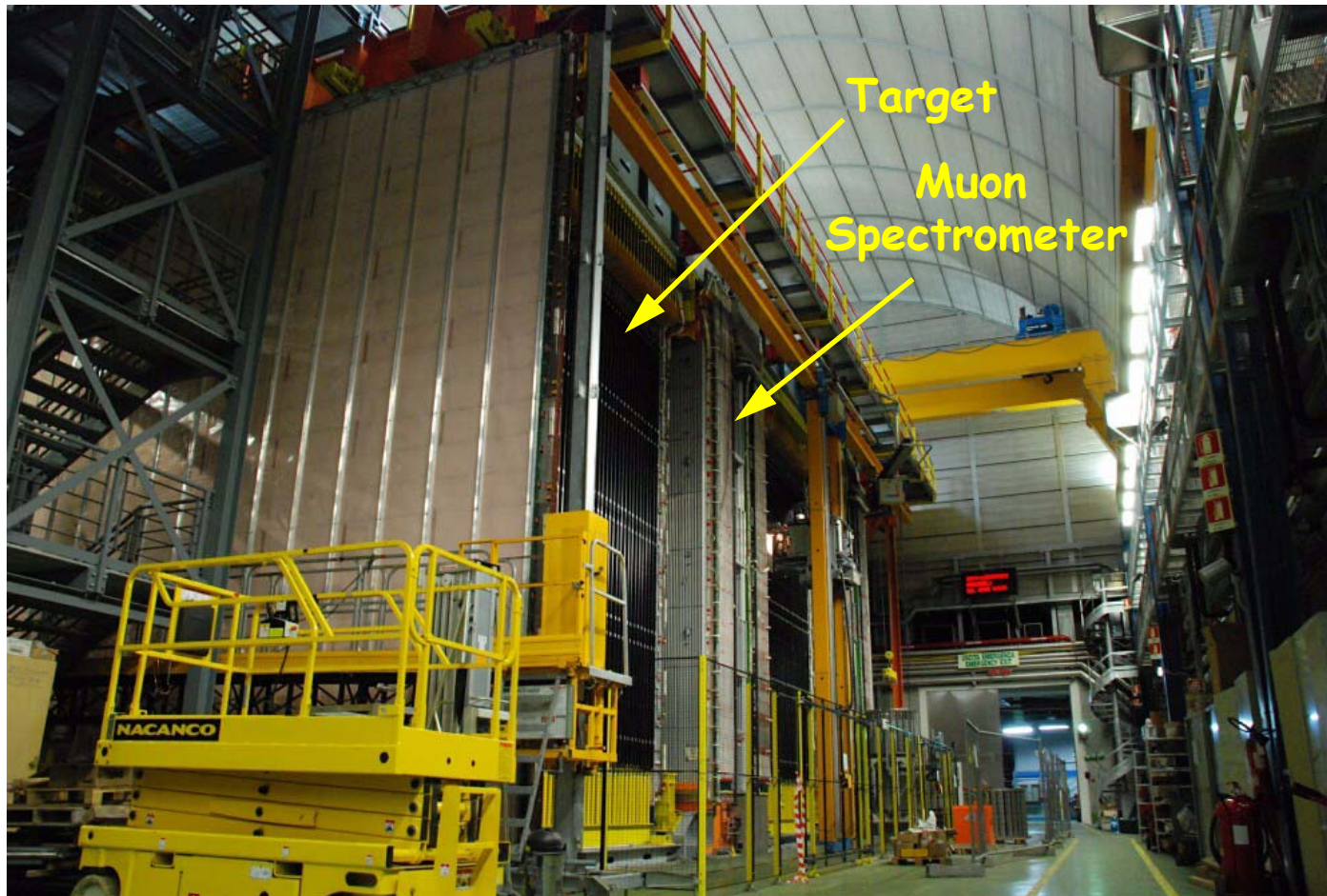
The Opera experiment down in its underground hall.
