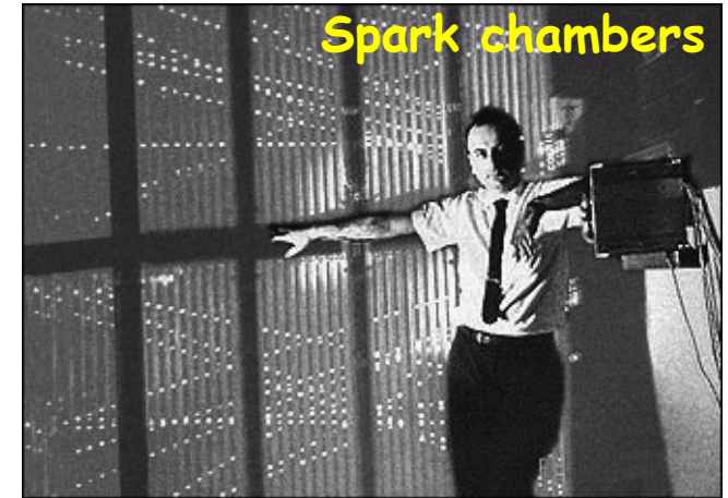
Sandwich of Aluminium plates and spark chambers
