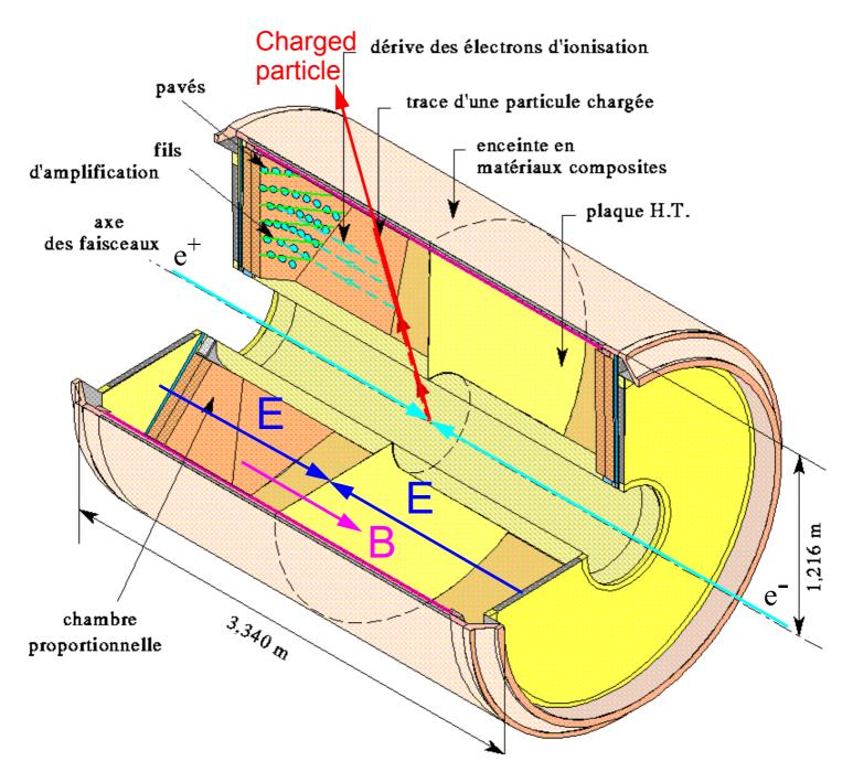
A charged particle ionize the gas in the cylinder and the electrons drift in an electrical field to the detectors at the ends of the cylinder.
