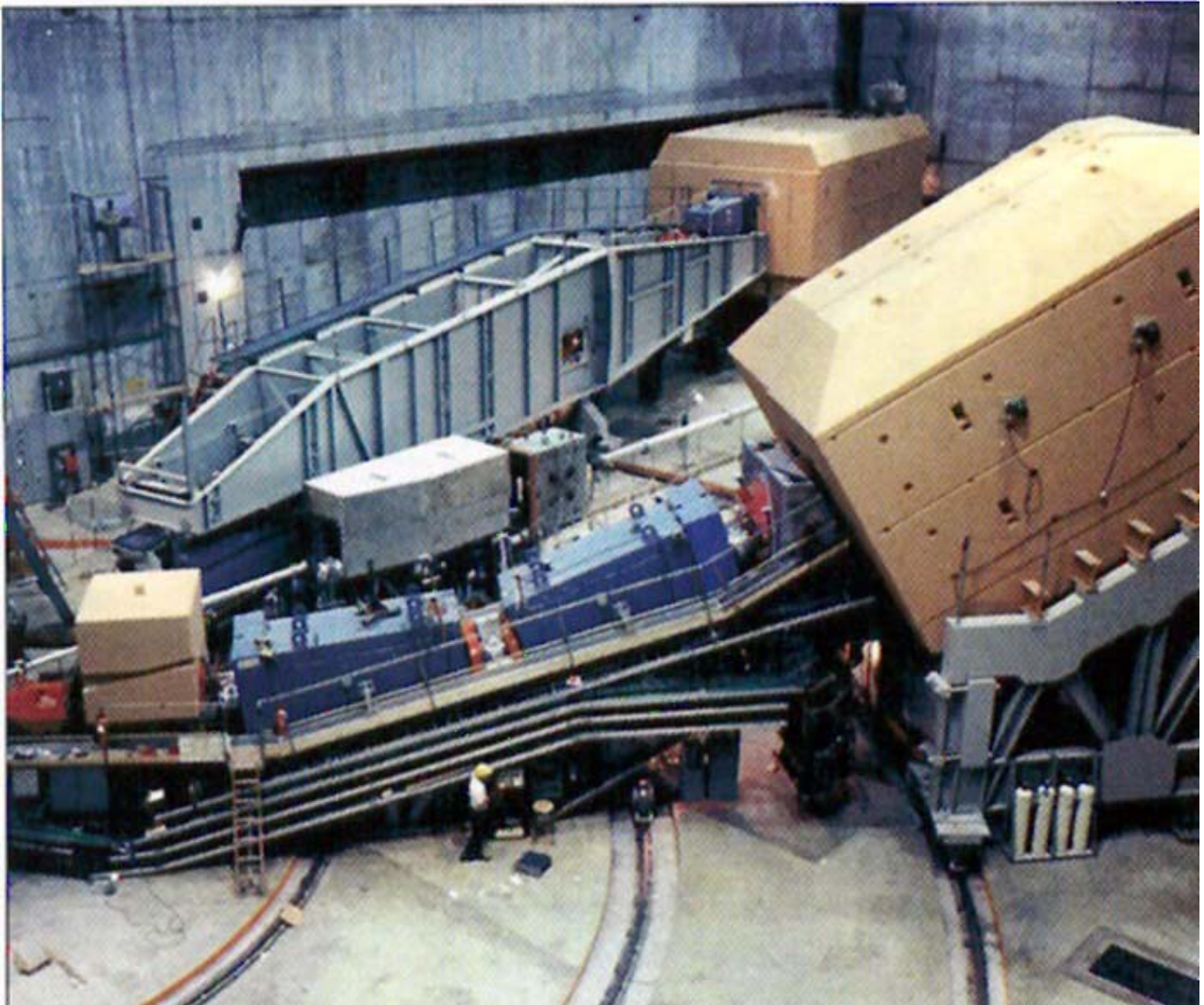
Figure 76: Two spectrometers in SLAC's End Station A that were used to discover quarks in the late 1960s.
